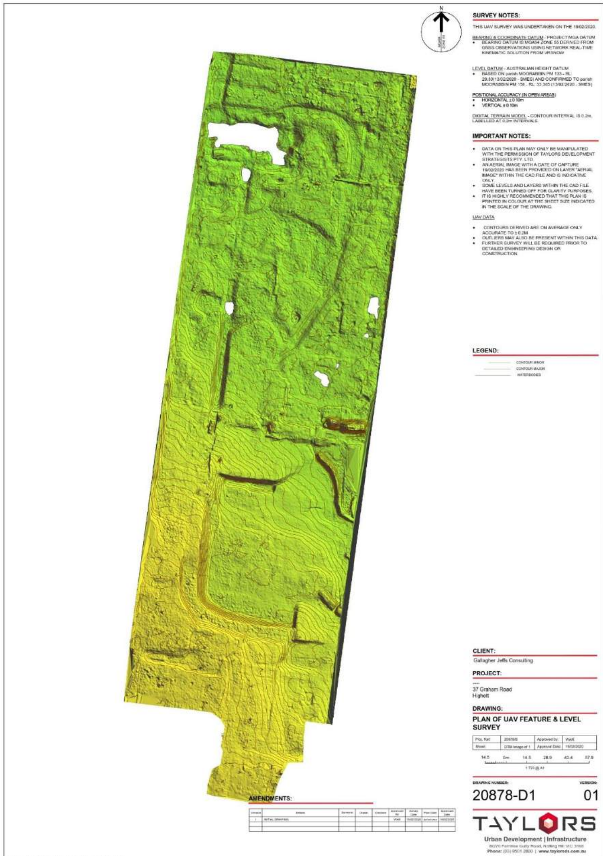
Figure 22: Digital elevation model February 2020 showing current ground levels across the activity area (provided by Gallagher Jeffs on behalf of the Sponsor)
